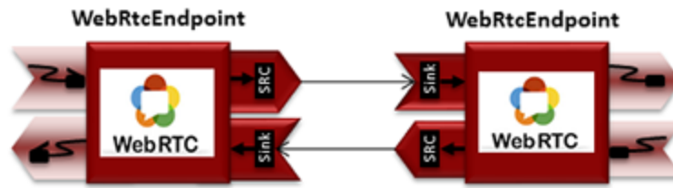
Fig. 33: One to one video call Media Pipeline
